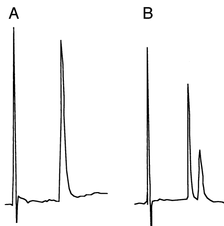
Fig. 4. LC-UV chromatograms of 25 \text{ g} of (A) Fetta cheese before and (B) after spiking with 8.24 \text{ ng g}^{-1} of roquefortine.
